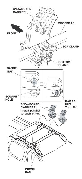
8. Turn the knobs on the top clamp to tighten the front carrier.
