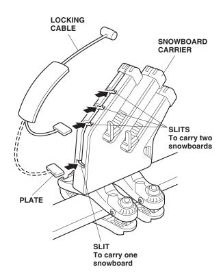
15. After loading the snowboards on the carrier, adjust them with the help of the board supports so that the top edges are level and the boards are as far down in the carrier as possible. To secure the snowboards, use the key to open the covers, and insert the locking cable barrels into the holes of the carrier covers.
